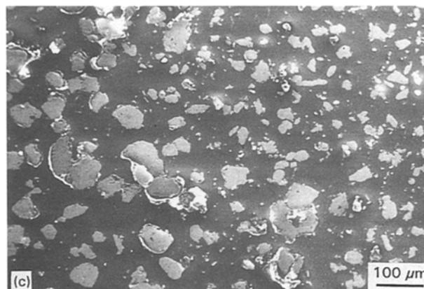
Figure 2 Nd-Fe-B particles size and morphology as a function of milling time: (a) 1 h, (b) 4 h and (c) 10 h.
