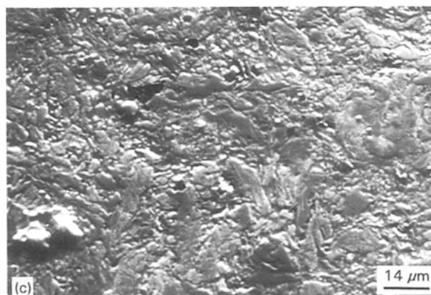
Figure 7 Microstructure of the Nd-Fe-B samples (a) before MA, and after mechanical alloying for (b) 4 h and (c) 12 h and subsequent annealing at 1023 K for 1 h.
