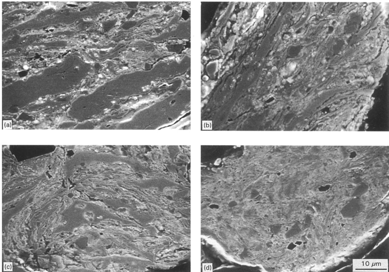
Figure 3 Microstructure of Nd-Fe-B powders mechanically alloyed for different times: (a) 1 h, (b) 4 h, (c) 6 h and (d) 10 h.
