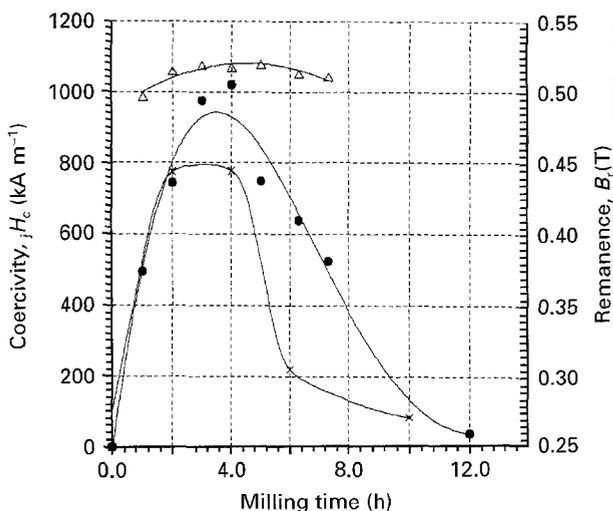
Figure 5 Dependence of coercive force (MA in (●) toluene and (×) argon) and (Δ) remanence on milling time for the powders annealed after milling at 1023 K for 1 h.
