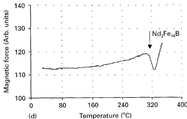
Figure 6 Magnetic force as a function of temperature for the samples before milling (i.e. only annealed) and after milling for 1, 4 and 12 h and annealing at 1023 K for 1 h.
