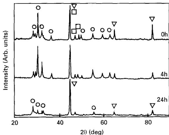
Figure 1 X-ray patterns of the Nd-Fe-B powders milled in toluene for different times. (○) Nd, (▽) Fe, (□)  $\text{Fe}_2\text{B}$ .
