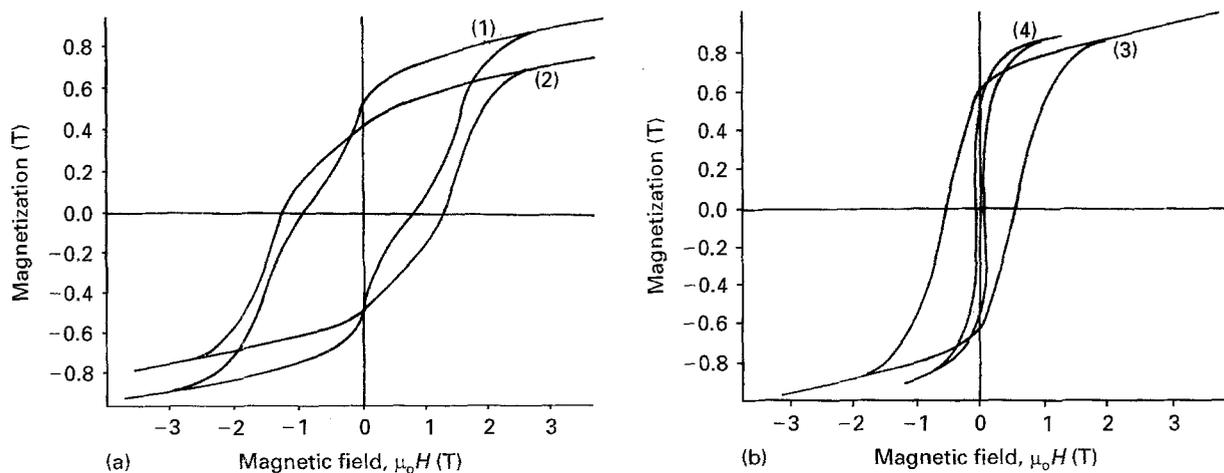
Figure 4 (a, b) Hysteresis loops for the powders milled for (1) 2 h, (2) 3 h, (3) 6 h and (4) 12 h and subsequently annealed at 1023 K for 1 h.
